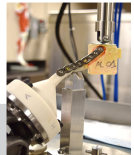
Fatigue loading of clavicle fracture plate
